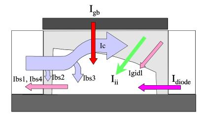
Fig. 3.1 Various current components inside the body.
