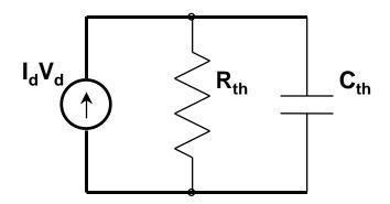
Fig. 5.1 Equivalent circuit for self-heating simulation.
