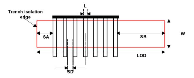
Fig. 9.3 Layout of multiple-finger MOSFET [27]
