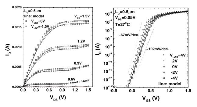
(Left) Fig. 6.2 The PD/FD transition can be captured by modeling  $\Delta V_{bi}$  [20].
