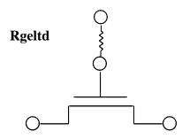
In this case, only the electrode gate resistance (bias-independent) is generated by adding an internal gate node. The electrode gate resistance Rgeltd is given by
