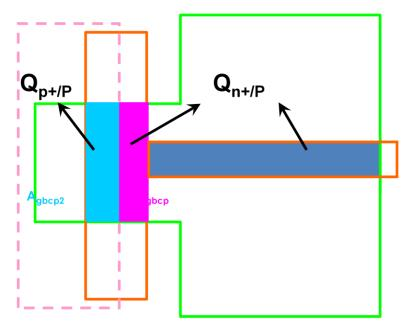
Fig. 4.5 The total charge in the opposite-type gate.
