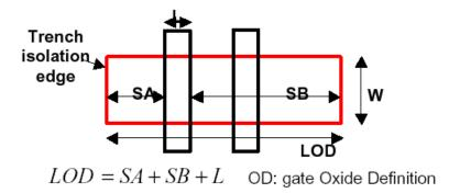
Fig. 9.1 shows the typical layout of a MOSFET [27]
