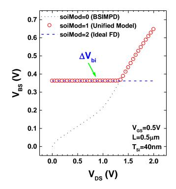
Fig. 6.1 The body potential in the unified model approaches the  $V_{BS}$  solved in BSIMPD for PD devices, while returns to  $\Delta V_{bi}$  for ideal FD devices [20].
