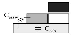
Fig. 4.2 SOI MOSFET extrinsic charge components.  $C_{essw}$  is the substrat<u>e</u>-to-<u>source sidewall capacitance</u>.  $C_{esb}$  is the substrat<u>e</u>-to-<u>source bottom</u> capacitance.
