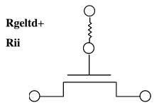
In this case, the gate resistance is the sum of the electrode gate resistance and the intrinsic-input
