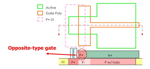
Fig. 4.4 Parasitic capacitance in opposite-type gate.
