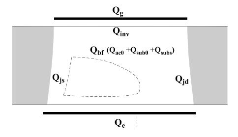
Fig. 4.1 Intrinsic charge components in BSIMPD CV model
