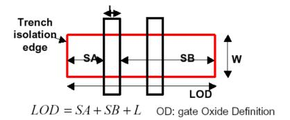
Fig. 9.1 shows the typical layout of a MOSFET [27]
