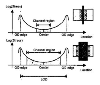
Fig. 9.2 Schematic stress distribution in the OD region [29]
