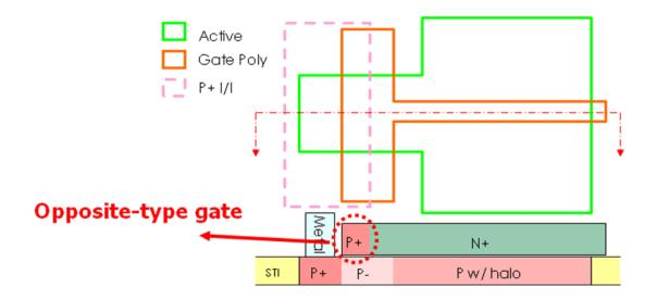
Fig. 4.4 Parasitic capacitance in opposite-type gate.
