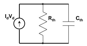
Fig. 5.1 Equivalent circuit for self-heating simulation.
