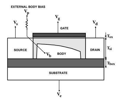
Fig. 2.1 Schematic of a typical PD SOI MOSFET.
