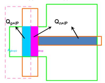
Fig. 4.5 The total charge in the opposite-type gate.
