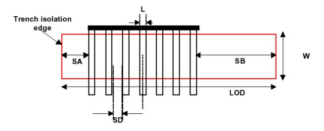
Fig. 9.3 Layout of multiple-finger MOSFET [27]
